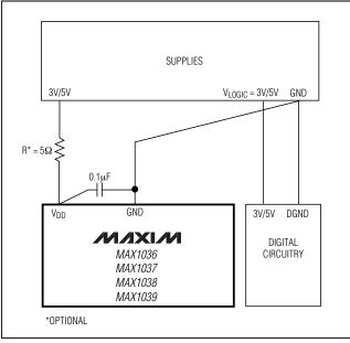
Figure 14. Power-Supply and Grounding Connections
