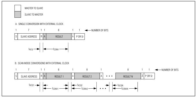
Figure 11. External Clock Mode Read Cycles
