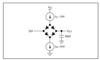
Figure 2. Load Circuit
