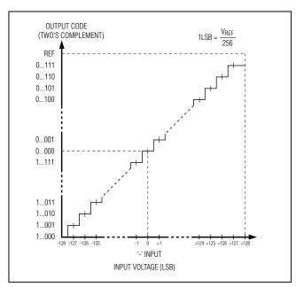
Figure 13. Bipolar Transfer Function
