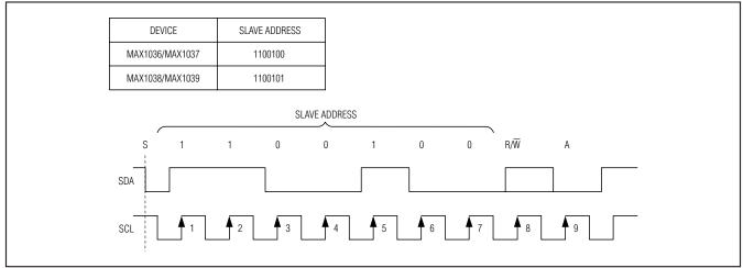
Figure 7. MAX1036/MAX1037 Slave Address Byte
