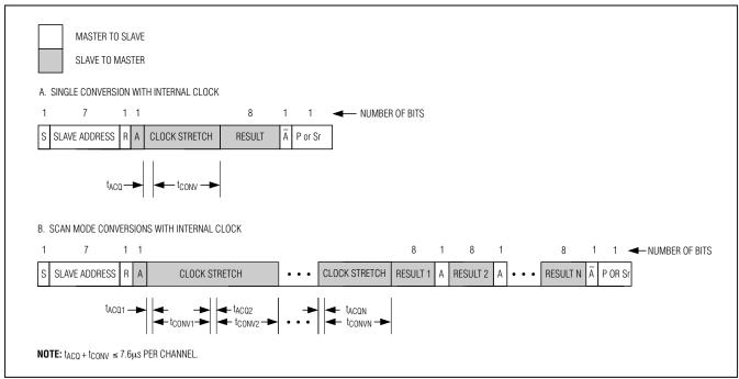
Figure 10. Internal Clock Mode Read Cycles
