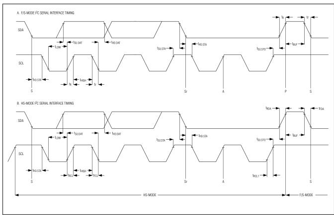
Figure 1. I<sup>2</sup>C Serial Interface Timing
