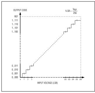
Figure 12. Unipolar Transfer Function
