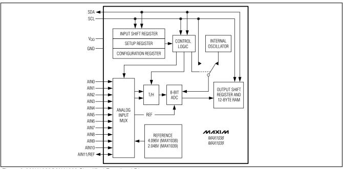
Figure 3. MAX1038/MAX1039 Simplified Functional Diagram
