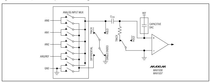
Figure 4. Equivalent Input Circuit
